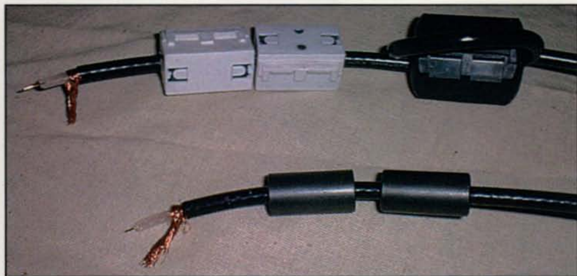
Photo E— Some common examples of ferrite beads used as RF chokes.
