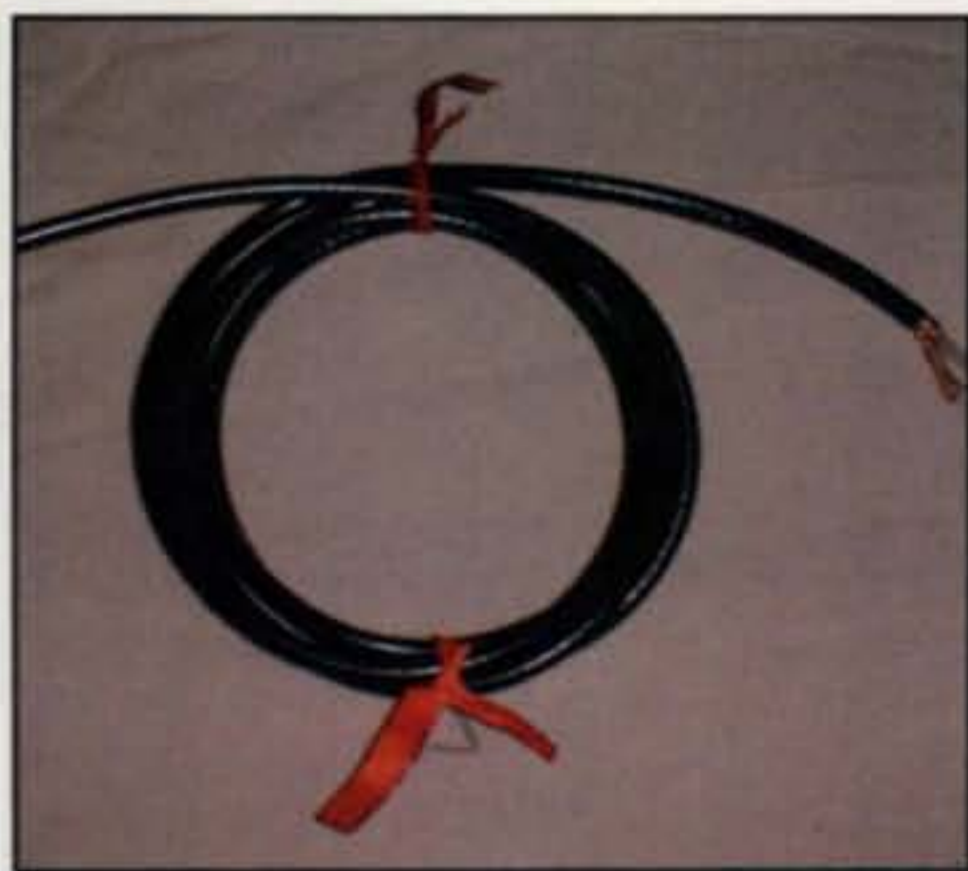
Photo F— If you don't have ferrite beads handy, several turns of coax will have a similar effect, creating what's known as a “noise balun.” (See text for details.)
